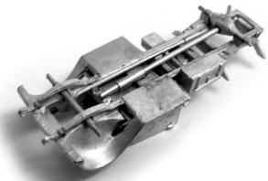
Set the front and rear axles in place. The rear diff will fit better one way round than the other - dry fit it to ensure you have it the correct way round - recess for the prop facing forwards.
